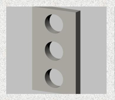
**ELECTROETCH DIM A ON EDGE OF SPACER**
